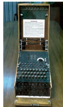
The Enigma machine, used by the German army to encrypt and decrypt messages during WWII, uses a dynamic letter scrambling technique.
